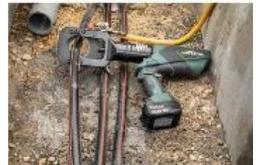
*Guillotine cable cutter Ø65mm - remote cutter with remote control for the BT network*
