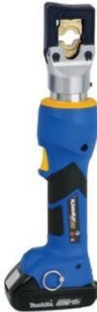
Hydraulic battery crimping tool 6 - 150 mm<sup>2</sup>.
