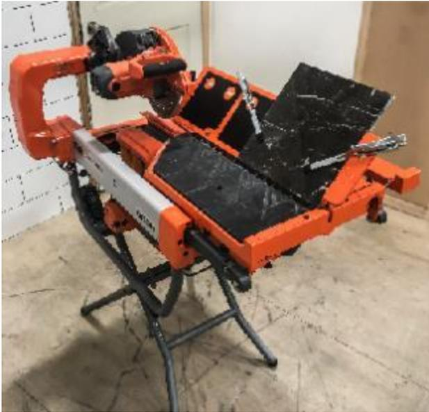
*A dust-free tiler's table saw that cuts cleanly, efficiently and precisely, without water, without mud, while keeping the blade cool.*
