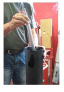
Insert centring bit into the wood hole saw.
